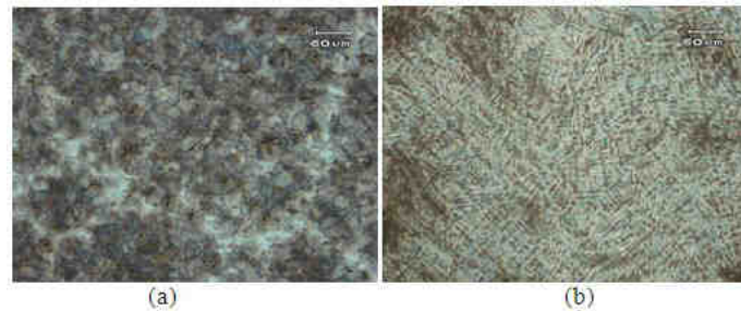
Figure 6. Micrograph at the thick wall (A) and at the tip (B), etched with Nital 3%.
